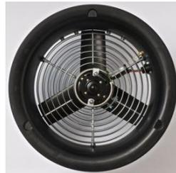
Abb. 6.24: BlowerDoor DuctBlaster (MiniFan)
